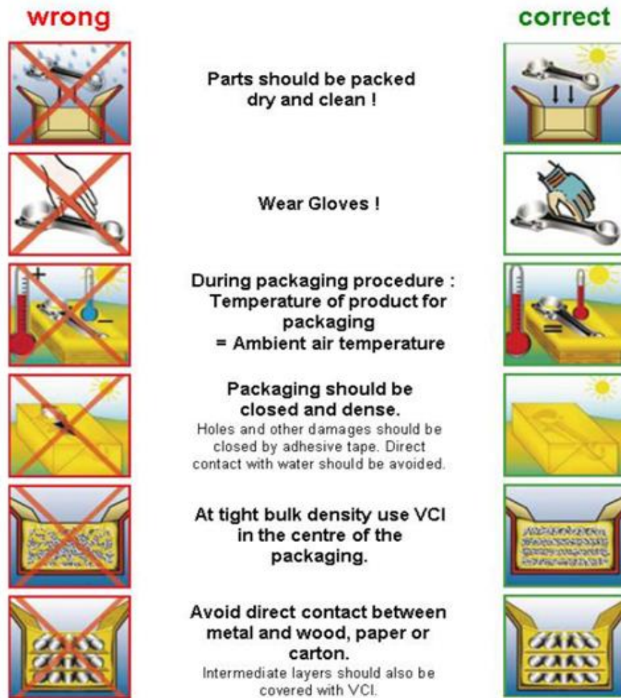
Figure 4: Methods of Application for Corrosion Prevention
