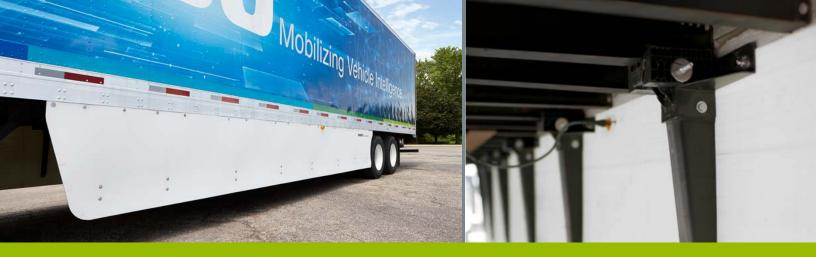
OptiFlow™ TrailerSkirt™ offers more than 5% fuel savings at US highway speeds (65 mph) and is EPA SmartWay and C.A.R.B. approved. TrailerSkirt reduces CO<sub>2</sub> emissions by up to 4.6 tons per trailer per year.
