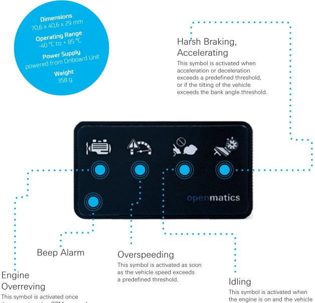
the current engine RPMs exceeds the preset engine speed threshold. is not moving for a predefined period of time.
