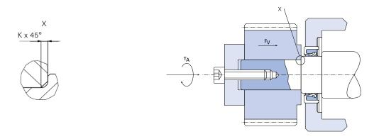
The connecting part on the gearbox output shaft must have a chamfer "K" (see table) on the contact pattern to the gearbox.
