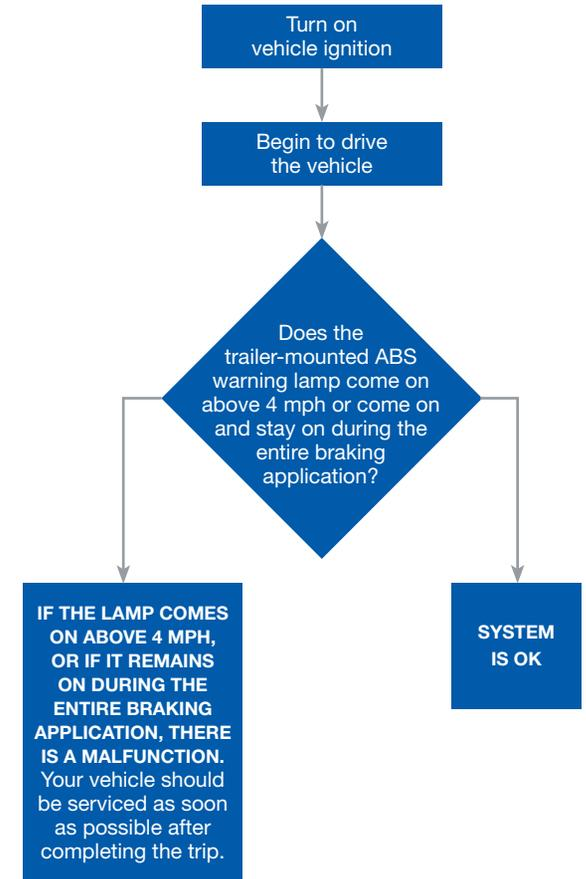
**Note:** Depending how the ABS is powered, the lamp may come on briefly at ignition and then go off, or briefly flash each time you apply the brakes on a moving vehicle.
