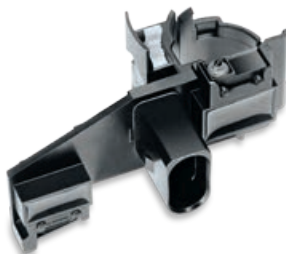
Component carrier with insert molded stamping grid for the three-dimensional configura- tion of micro-switches on the trunk lock cylinder
