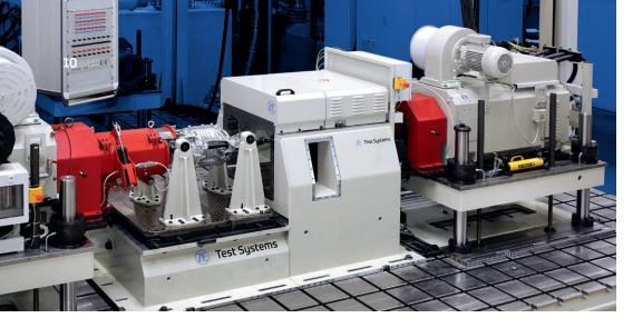
E-mobility test system up to 750 kW / 1,200 Nm torque for e-motors, gearboxes, e-axles, e-powertrain, e-transmissions.
