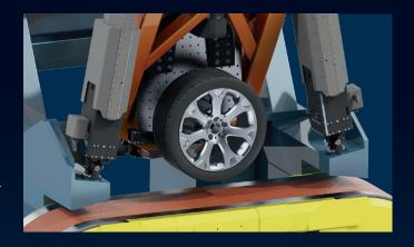
The Road Belt Tester ZF-RB 5 has remarkable advantages for demanding measurement tasks:
