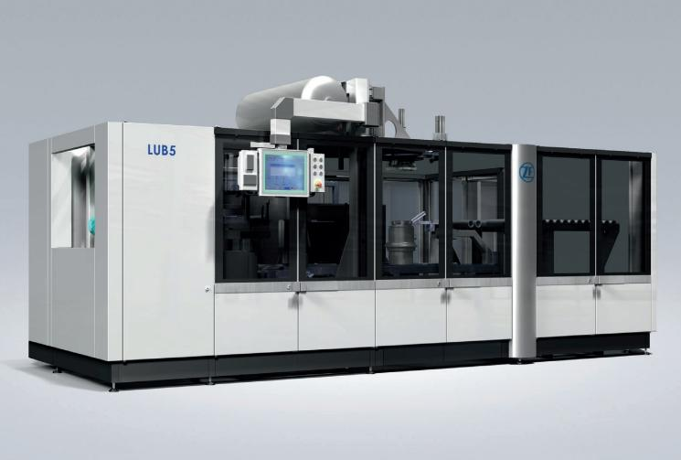
**ZF-LUB5:** Low Speed Uniformity and Balancing technology combined in one system.
