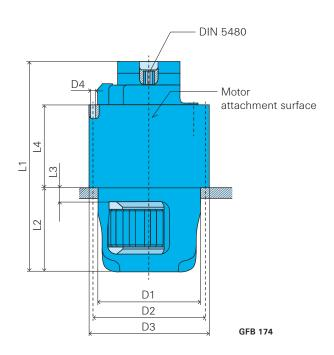
X = The gearing of the output pinion (module, number of teeth, tooth width, etc.) is determined by the customer's ring gear.
