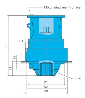
X = The gearing of the output pinion (module, number of teeth, tooth width, etc.) is governed by the customer's ring gear.
