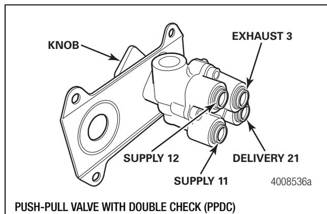
PUSH-PULL VALVE WITH DOUBLE CHECK (PPDC)
