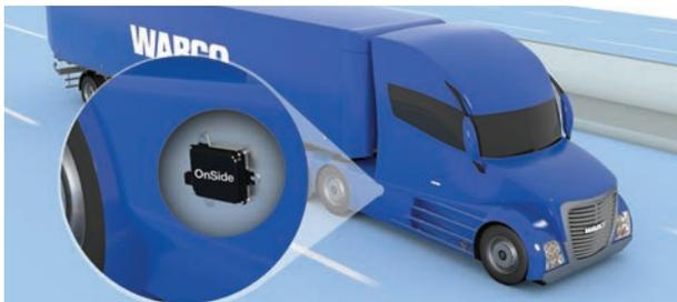
This Driver Tips Guide applies to vehicles equipped with WABCO OnSide™ Blind Spot Detection System. OnSide is a radar-based warning system that assists drivers in checking adjacent lane clearance before merging. When used in conjunction with proper lane changing procedures, this system can reduce the risk of accidents. Please read the following information to operate the system properly and understand the system's support as well as situations in which this system may not provide assistance.
