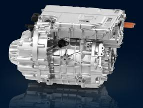
The ZF Electric Axle Drive features an integrated e-drive system with e-motor, power electronics and reducer for a compact design. Now, ZF Aftermarket is introducing a range of 43 repair kits to help you get your customers back on the road.
