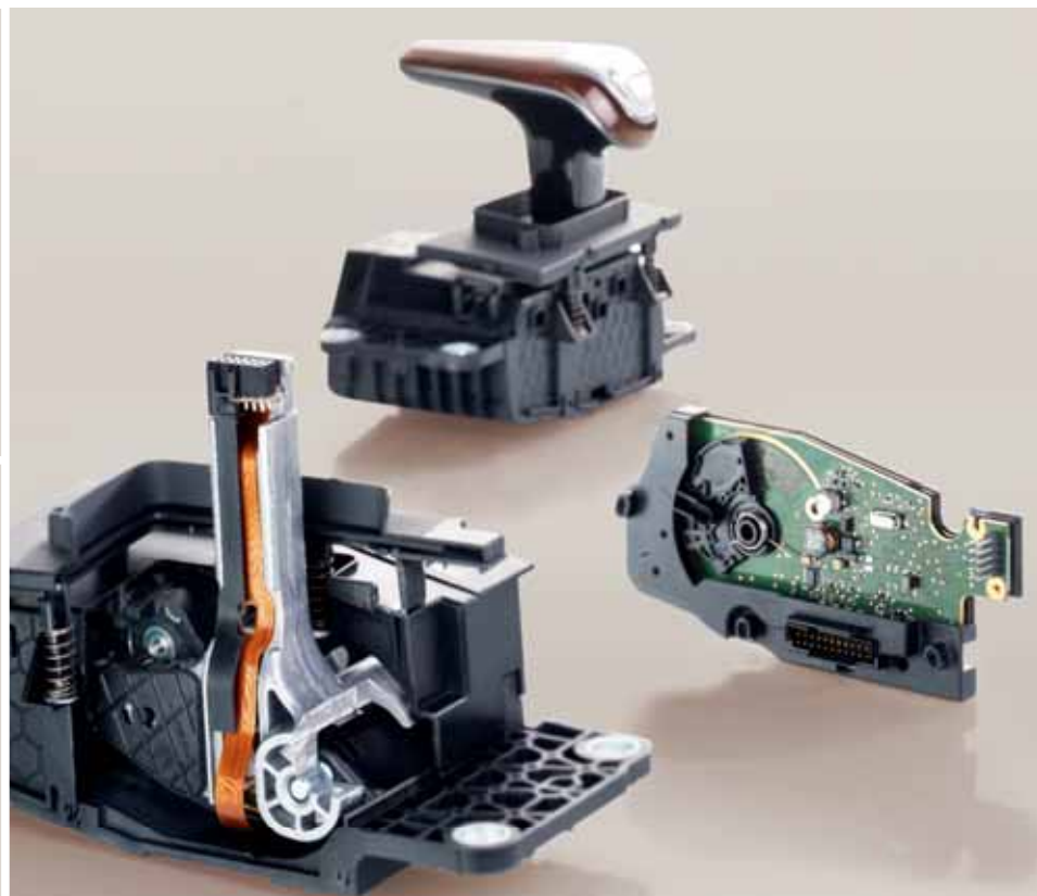
Shift-by-wire gearshift for automatic transmissions
